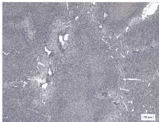
Fig. 6 Optical micrograph of ingot-cast IN-738 at ( M_o ) = 800 \times
