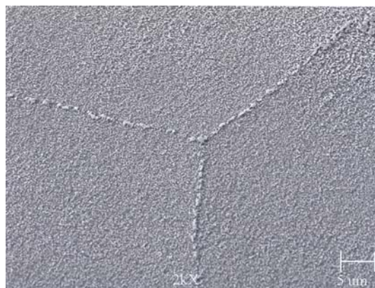
Fig. 8 Electron micrograph of the wrought condition for ingot-cast IN-738 after extrusion at ( M_0 ) = 2000 \times
